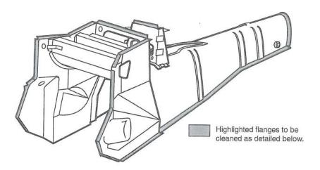
The early MGB (1962-67) and MGB GT (1965-67) utilised a three synchro gearbox which was different in shape to the later four synchro boxes (fitted until the end of MGB production in 1980). The tunnel assembly surrounding the early gearboxes was substantially different from the later units.
